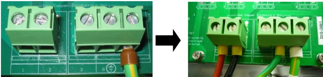
Figure 7.2.6: Connect the AC Cables to Correct Positions
