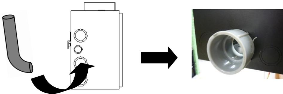
Figure 7.2.3: Insert a conduit through an open hole
