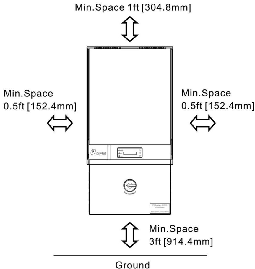
Figure 5.4.2: Required Clearance Space
