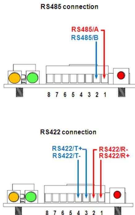
Figure 6.2.4: RS 485/RS422 connections
