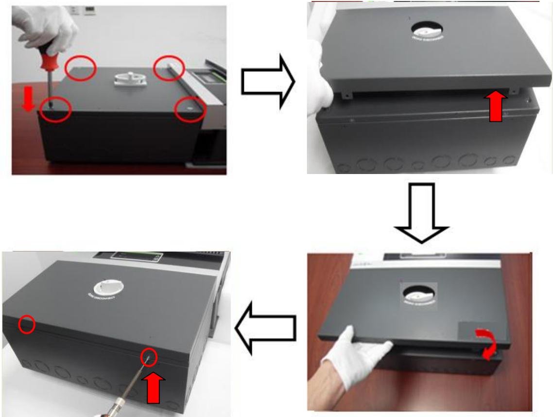
Figure 7.2.7: Reinstall the top cover of wiring box
