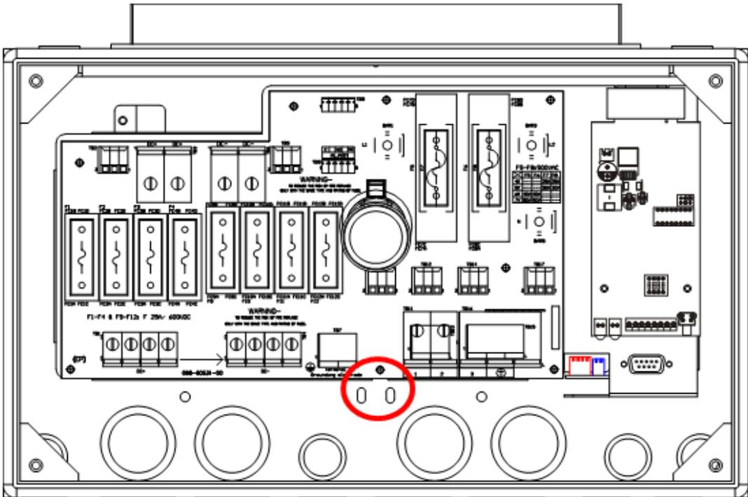
Figure 5.4.11: Screwing Location for the Security Screws
