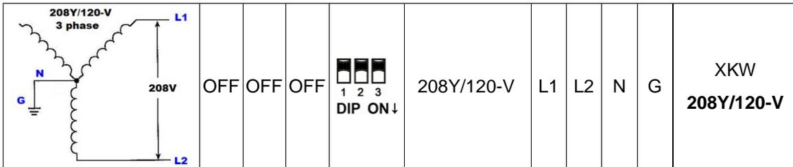
Note: The neutral conductor is required to be the same gauge as the phase conductors.
