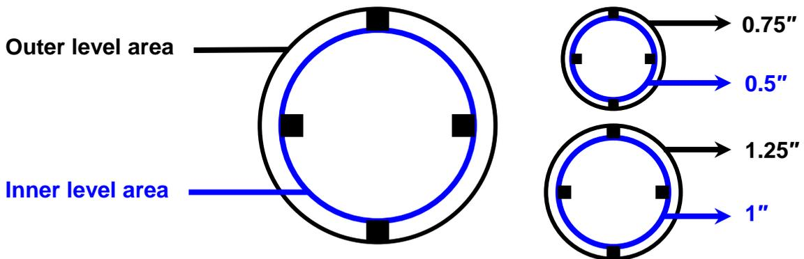
Figure 6.4.3: Levels area and the size of Knockouts
