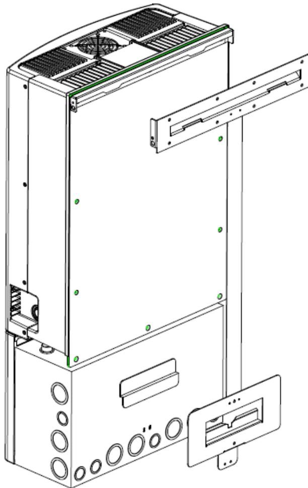
Figure 5.4.7: Install PV Inverter into mounting bracket
