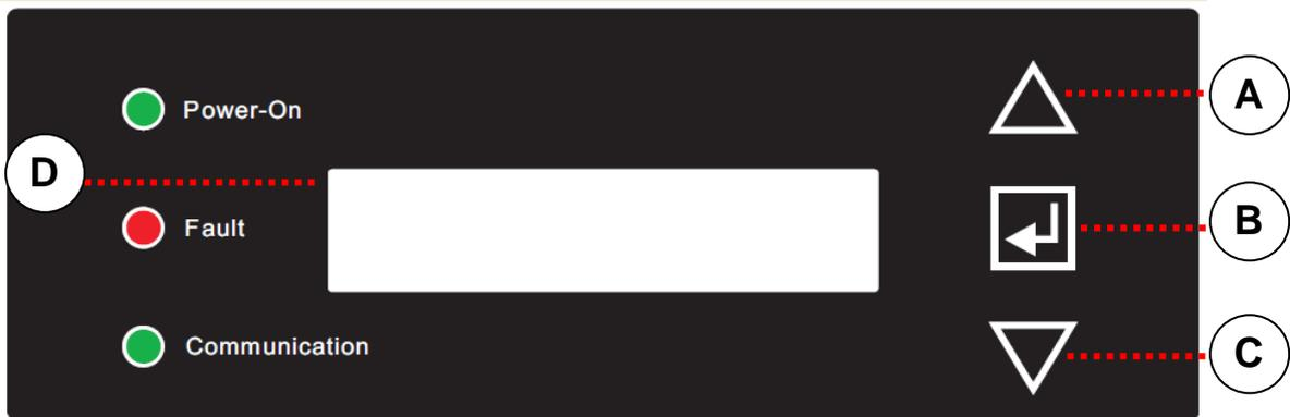
Figure 4.6.1: Control buttons and LCD displays
