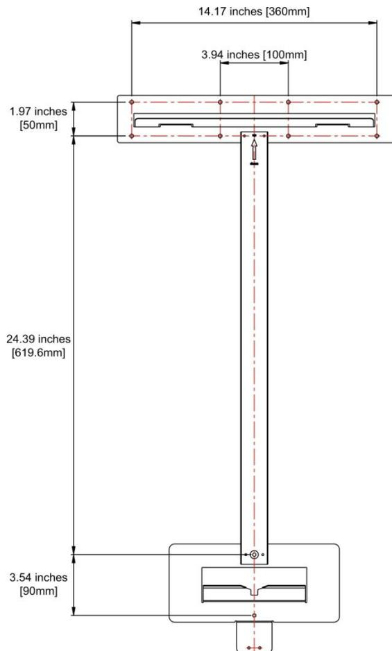
Figure 5.4.4: Dimension of Drilling Point for the Wall
