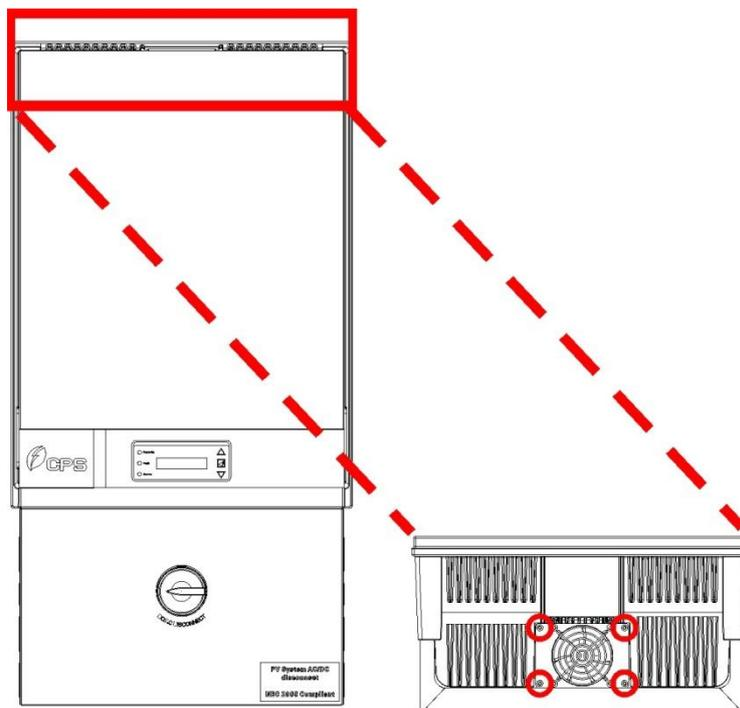
Figure 9.1.2: Screws for the external cooling fan
